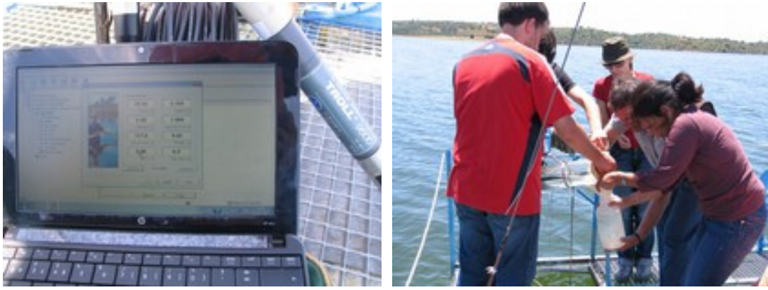
Figure 3.15 The TROLL 9500 multi parametric probe (left). Collection of water samples with the Van Dorn bottle.
