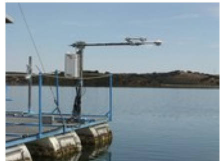
Figure 3.9: Albedometer and pirradiometer
