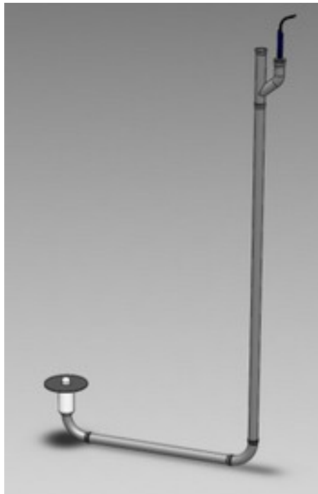
Figure 7.1 Schematic representation of the Underwater Solar Irradiance Profiler
