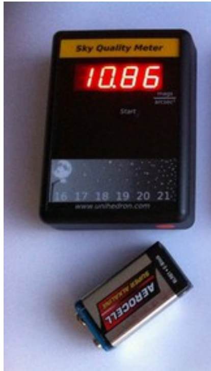
Figure 3.26 Unihedron Sky Quality Meter-L
