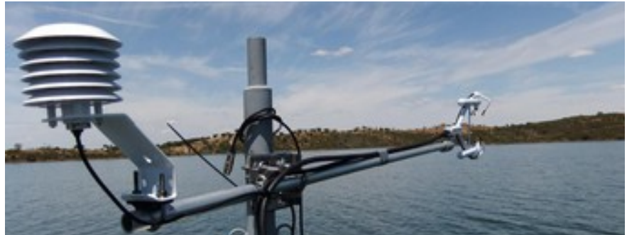
Figure 3.11: View of the eddy correlation system
