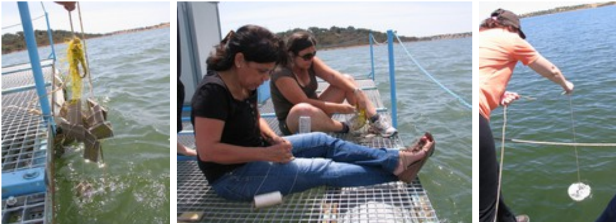
Figure 3.16 Collection of diatoms from the artificial substrates placed in the platform Alqueva-Montante (left and center). Measuring the Secchi disc depth (right)
