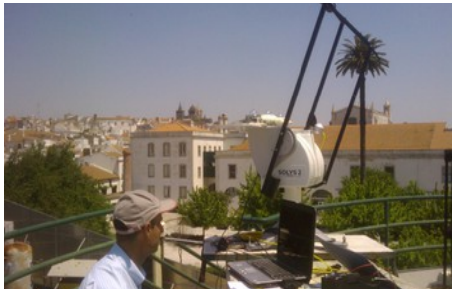
Figure 2.19 Test of the sun tracker and pyranometers calibration (17/05/2014)
