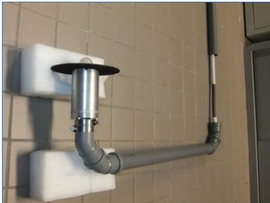
Figure 7.2 Multi-layers frame developed to protect the optical cable (not visible here) and the optical receiver with a field-of-view (FOV) of 180°
