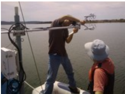
Figure 3.7: Mounting the eddy correlation system
