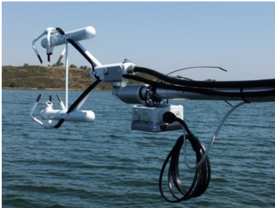
Figure 2.23 Case containing the accelerometer attached to IRGASSON system mounted on a raft.
